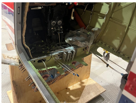
Where's the floor? Removed to replace the landing gear brackets
